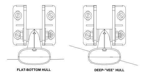
NOTE: Some aluminum boats with strakes or ribs on the outside of the hull create large amounts of turbulence at high speed. These boats typically have large outboard motors capable of propelling the boat at speeds over 35 mph. The transducer should be mounted as far below the hull as possible on these boats. This will place the face of the transducer below the turbulent water, allowing the sonar unit to work at high speeds.
